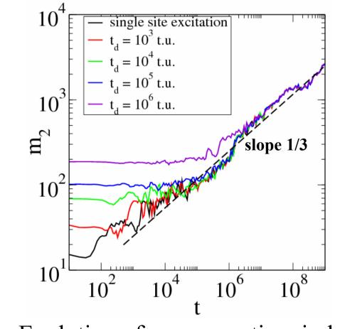
Evolution of  $m_2$  versus time in loglog plots. Single site excitation in the intermediate regime II for the KG model corresponds to the black curve. The wave packet after  $t_d = 10^3$ ,  $10^4$ ,  $10^5$ ,  $10^6$  time units (t.u.) is registered and relaunched as initial distribution.
