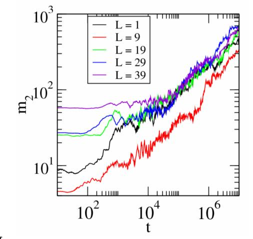
Nonlocal excitations of the KG chain corresponding to initial homogeneous distributions of energy E=0.4over L neighboring sites.  $m_2$ versus time in log-log plots for L=1, 9, 19, 29 and 39 sites.
